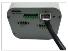
If necessary, connect the other external devices, such as DI/DO, PT scanner or power adapter to the camera. See *Before Installation* on page 13 for more information.
