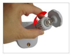
3. Screw the camera to the bracket.
