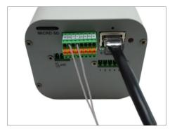
Connect the other end of the network cable to a switch or injector. Then, connect the switch
