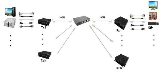
Multiple TX to One RX r Connection: (KVM Switcher over IP)
