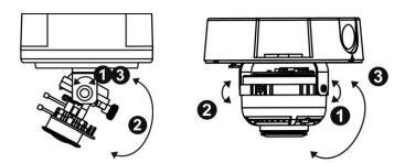
iii. Release the video adjustment screw and then adjust the lens direction. After completion, tighten the video adjustment screw.
