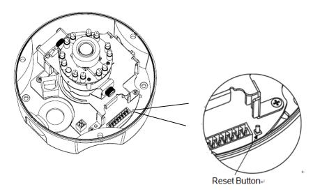
The Reset Button can be used to reboot the camera, restore it to factory default settings, or switch on FocusEasy. If the camera experiences a problem, rebooting the camera may correct the problem. If the problem remains, please restore the camera to factory default settings and reinstall the software.
