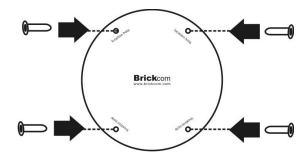
4) Mount the camera on the wall and position to two screw slots over the plastic anchors. Insert the screams into the holes and use the screwdriver to tighten the screws clockwise until they are secure.
