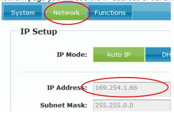
You could also input the IP address of transmitter / receiver at link column of browser if you know the exact IP address of them.
