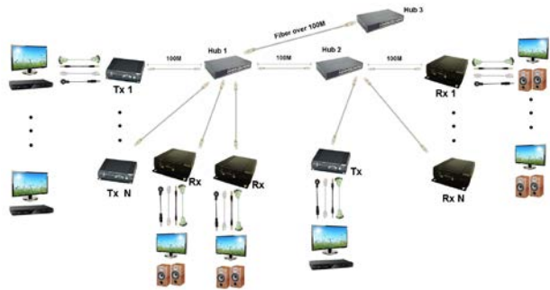
Multiple TX to Multiple RX via Switch Hub Connection
