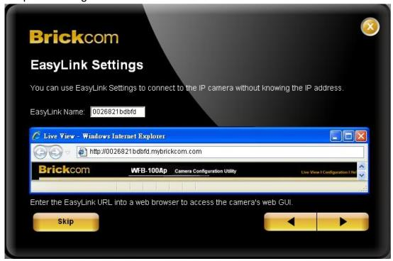
EasyLink<sup>TM</sup> is a unique Brickcom function which allows users to assign a unique EasyLink name to their network camera's IP address. There is no need to configure the router to open up ports or remember hard-to-memorize IP addresses. Users can log onto [uniqueEasyLinkname].mybrickcom.com to view the camera's web GUI and live view.
