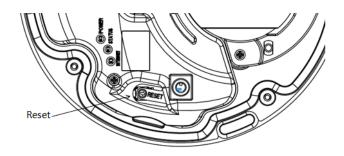
The Reset Button can be used to reboot the camera or restore it to factory default settings. If the camera experiences a problem, rebooting the camera may correct the problem. If the problem remains, please restore the camera to factory default settings and reinstall the software.
