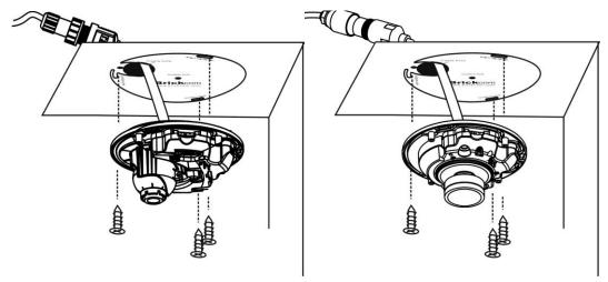
8. If you use the Mounting Adapter, please use the three screws which are included in the product package and a screwdriver. Mount the camera on the wall or ceiling and position the three screw slots over the plastic anchors. Insert the screws into the holes and use the screwdriver to tighten the screws clockwise until they are secure.
