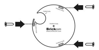
5. Hammer the three plastic anchors which are provided in the product package into the three location holes.
