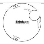
4. Drill three holes through the center of the three location holes on the sticker.
