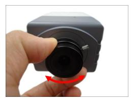
2. If necessary, tighten the lever screw to fix its position to avoid moving the lens.
