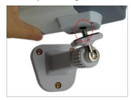
4. Tighten the hand knob until the camera is secured to the bracket.
