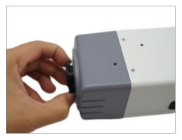
3. Twist and pull to remove the cap covering the threaded end of the lens.
