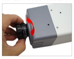
2. Twist and pull to remove the cap from the threaded end of the replacement lens.
