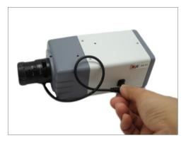
5. Pull to remove the protective cap from the replacement lens.
