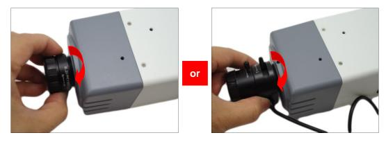
5. For cameras models D2xVA, E2xVA, E2xA, and E270, connect the lens cable to the DC-iris port.
