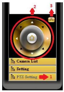
On the PTZ control section, click the arrow (marked by **3** on the picture) for the **Preset Point and Patrol** section to come up.
