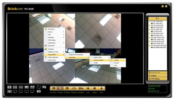
On the BRC64 PC-NVR, you can use the mouse or the software control panel to perform the PTZ (pan, tilt, zoom) operations. For the mouse-based PTZ control, the drag operation of the mouse changes the viewing direction, and the mouse wheel does the zoom-in and zoom-out of the image.
