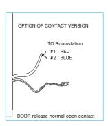
4. If there is no hole on the wall, you can allocate the wire on the groove around the case as appeared in the figure.
