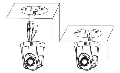
E. Turn the PTZ camera counter clockwise until it is in a locked position.
