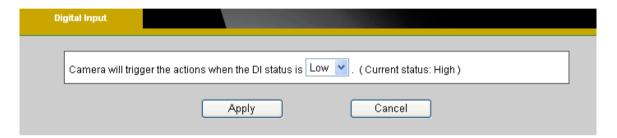
The DI socket allows the IP camera to receive input from an external device. The external device should have the ability to drive voltage on the connected DI wire to the triggering voltage level in order to notify the IP camera of any event of interest. The IP camera will then process the event notification according to the specific event rules.
