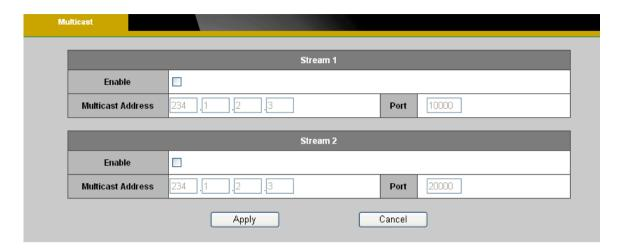
Multicast sends a video stream to the multicast group address and allows multiple clients to acquire the stream at the same time by requesting a copy from the multicast group address. Therefore, multicast can effectively save Internet bandwidth. The RTSP (Real-Time Streaming Protocol) controls the delivery of streaming media.
