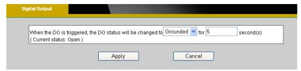
The DO socket allows the IP camera to send output to an external device. While executing the DO notification action, the IP camera drives voltage on the connected DO wire to the triggering voltage level for X number of seconds. The connected external device will then be triggered for X number of seconds.
