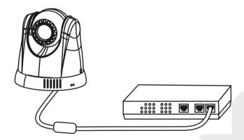
Use a single Ethernet cable to connect the camera to the High Power PoE-enabled switch.
