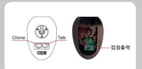
After opening the cover of the stand bottom, connect the Receiver or the Remote Chime for the system to the 2P terminal block.
