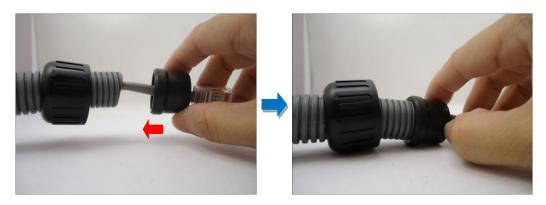
**Step 3: Install the Ethernet Cable**
