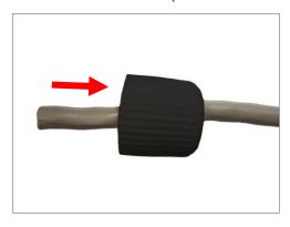
4. Insert the cable through the gland body.
