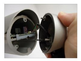
3. Remove the pre-installed cable gland and network cable using a wrench (not included in the package).
