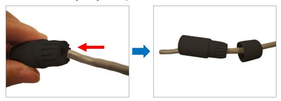
5. Attach the RJ-45 connector to the cable. For pin mapping and detailed instructions, see *How to Attach the RJ-45 Connector* on page 29 for detailed information.
