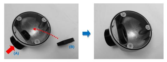
2. Insert the Ethernet cable through the back cover and then align the sealing insert to the gland body.
