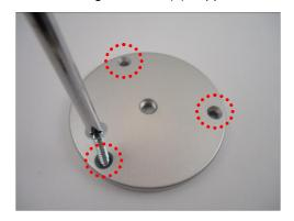
3. Attach the bracket to the plate.
