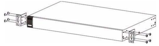
**2** Using a #2 Philips screwdriver, install the M3 flat head screws through the mounting bracket holes into the Switch.
