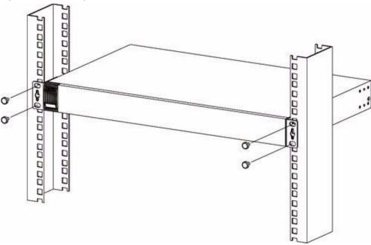
Figure 9 Mounting the Switch on a Rack (ES1100-24)
