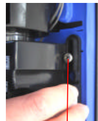
Loosen the four unit base mounting screws
