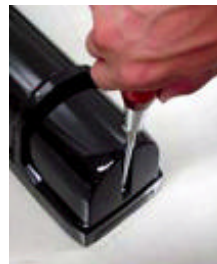
Loosen a cover lock screw
